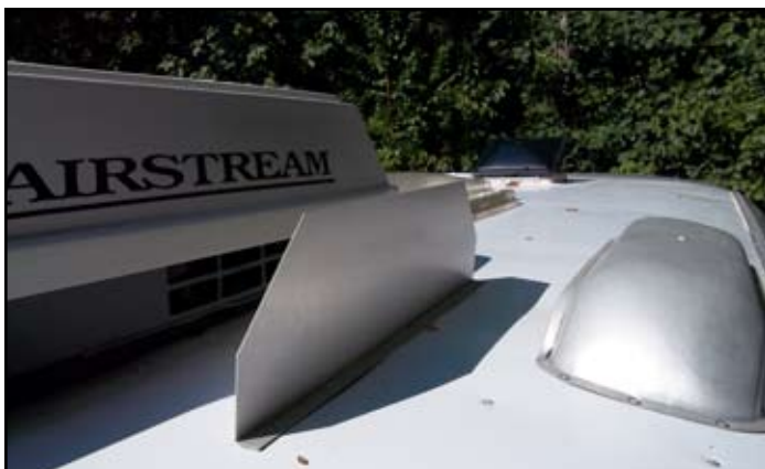
Left to right: air conditioner, baffle, and the refrigerator vent.
